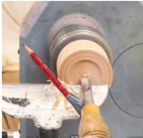
STEP 14. You can clearly see the flute position of the tool here. The pencil (which is in line with the flute) shows that the tool is being presented at around 10 o'clock – a good safe place to make the cut
